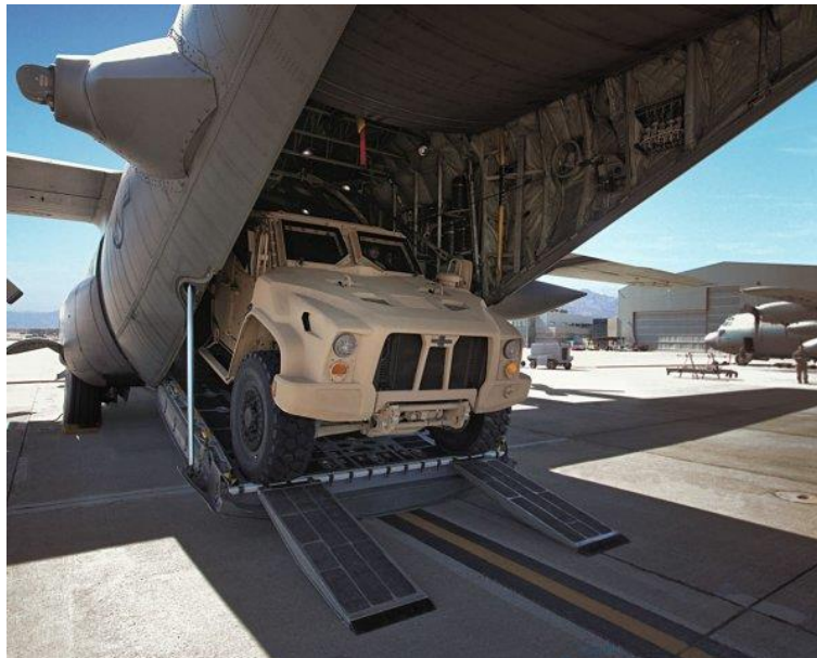
Oshkosh Defense's JLTV is air-transportable by Lockheed C-130 Hercules transport aircraft. The vehicle shown during trials is in GP configuration (Oshkosh)
