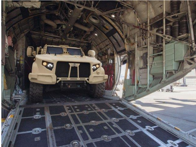
Oshkosh Defense's JLTV is air-transportable by Lockheed C-130 Hercules transport aircraft. The vehicle shown during trials is in GP configuration (Oshkosh)
