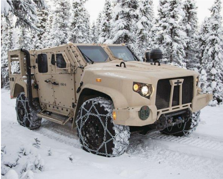
A USMC LRIP JLTV in M1280 GP (JLTV-GP) configuration; this vehicle is also fitted with a deep fording kit and tyre chains (Oshkosh)
