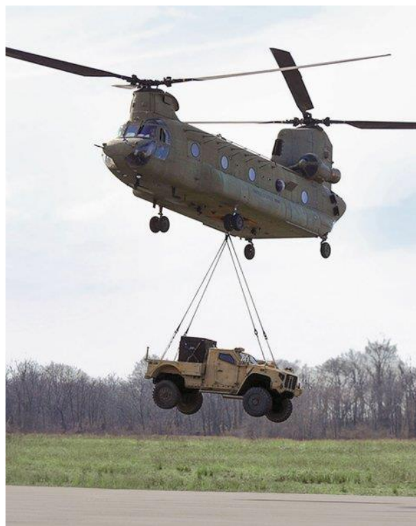
Oshkosh Defense's JLTV is transportable as an underslung load by CH-47 Chinook helicopter. The vehicle shown during trials is in Utility configuration (Oshkosh)
